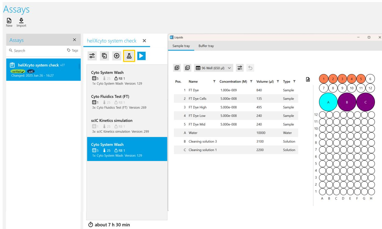
2. Put buffer in the buffer tray and insert buffer lines 1 and 3 into the buffer, while leaving the line 2 in air. Click on the sample tray and insert the ready-to-use glass vials, as illustrated by the **heliOS Sample tray layout** (shown below).
