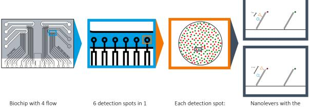
Biochip with 4 flow channels, each with multiple detection spots in series 6 detection spots in flow channel
