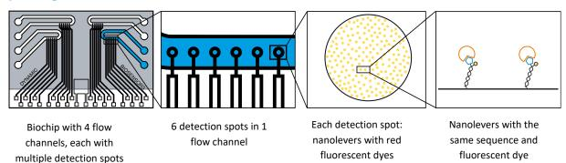
The detection spots are functionalized with one nanolever, either NL-CAS-B48 on probe spots or NL-CAS-A48 on reference spots. The 5'-end of the DNA is fixed on the surface while the 3'-end carries a yellow fluorescent dye (Y1).
