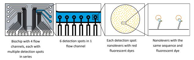
The detection spots are functionalized with one nanolever NL-B48. The 5'-end of the DNA is fixed on the surface while the 3'-end carries a yellow fluorescent dye (Y1).
