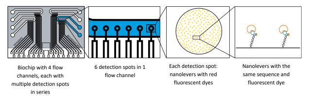
The detection spots are functionalized with one nanolever NL-B96. The 5'-end of the DNA is fixed on the surface while the 3'-end carries a yellow fluorescent dye (Y1).
