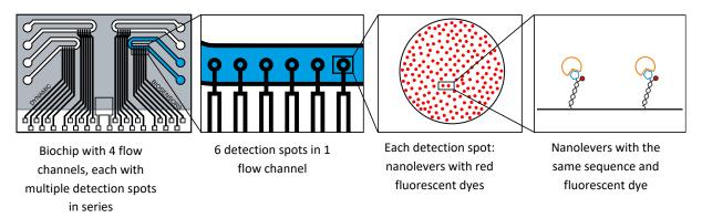
The detection spots are functionalized with one nanolever, either NL-B96 on probe spots or NL-A96 on reference spots. The 5'-end of the DNA is fixed on the surface while the 3'-end carries a red fluorescent dye (R1).
