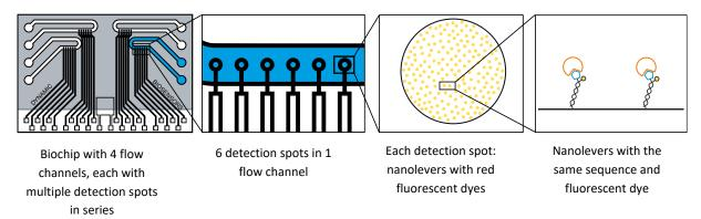
The detection spots are functionalized with one nanolever, either NL-B96 on probe spots or NL-A96 on reference spots. The 5'-end of the DNA is fixed on the surface while the 3'-end carries a yellow fluorescent dye (Y1).
